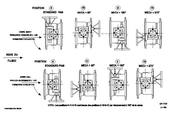
POSITIONS POSSIBLE DU MECANISME VANNE. OUVERTE PAR RAPPORT À LA NORME NE 29431 AVEC. COMMANDE À L'ENTREE. FAH. OU. FSH
