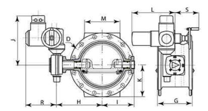
Standard version with short duty actuator S2-15 min, 400 V -3 - 50Hz, IP68.8, KN protection and heater 230 V.
