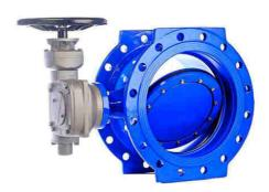
Flanged Butterfly Valve (flange-flange) with joint in the automatic butterfly (JPA) with double eccentricity and long spacing between the flanges.
